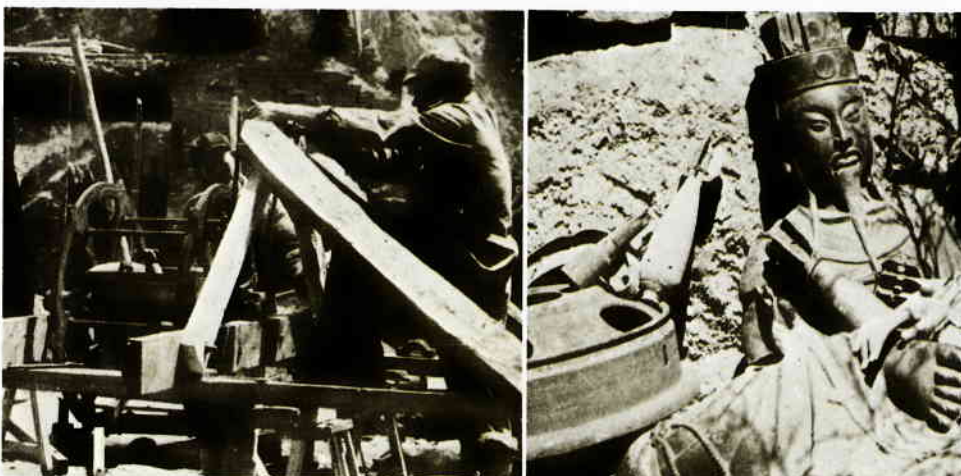
This Yan'an iron factory's furnace and water pump were ingeniously contrived from available materials such as a Buddha from an abandoned temple, 1949.
