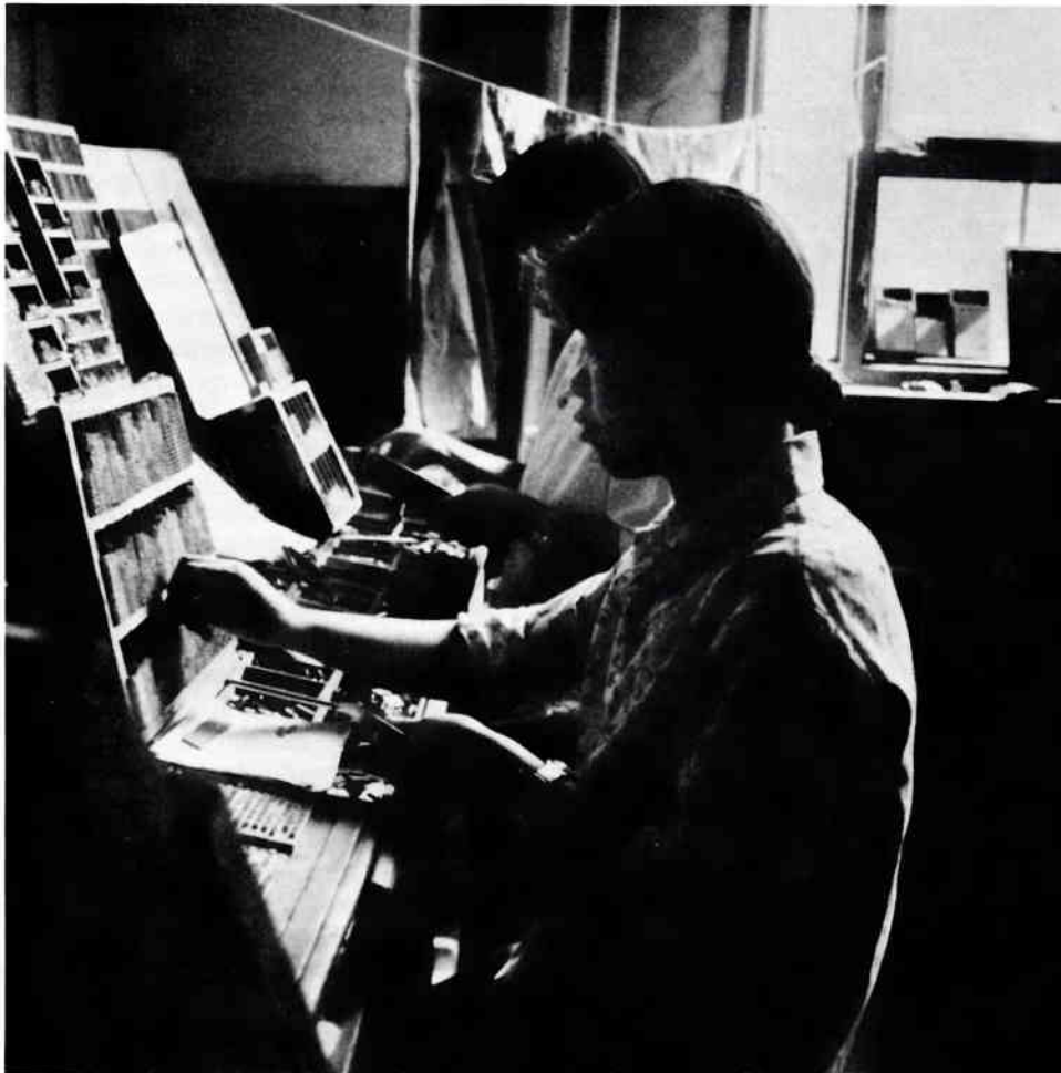
Because the written language employs thousands of characters, Chinese books have to be typeset by hand. (Photo: F. Levy)
