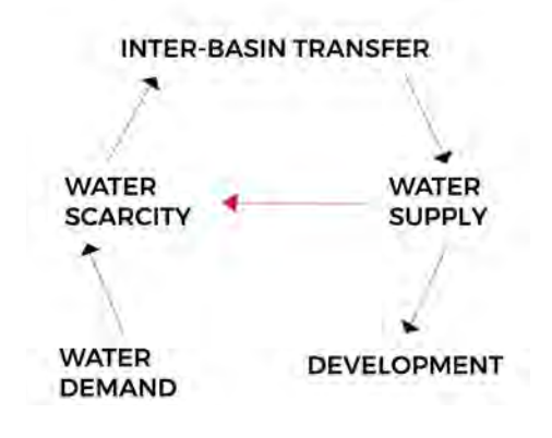
Figure 4: What I have previously called the 'universal truth': interbasin transfers increase the supply of water in the recipient region, but that supply creates the conditions for further development, which, in turn, raises demand. As demand continues to grow, scarcity reappears.
