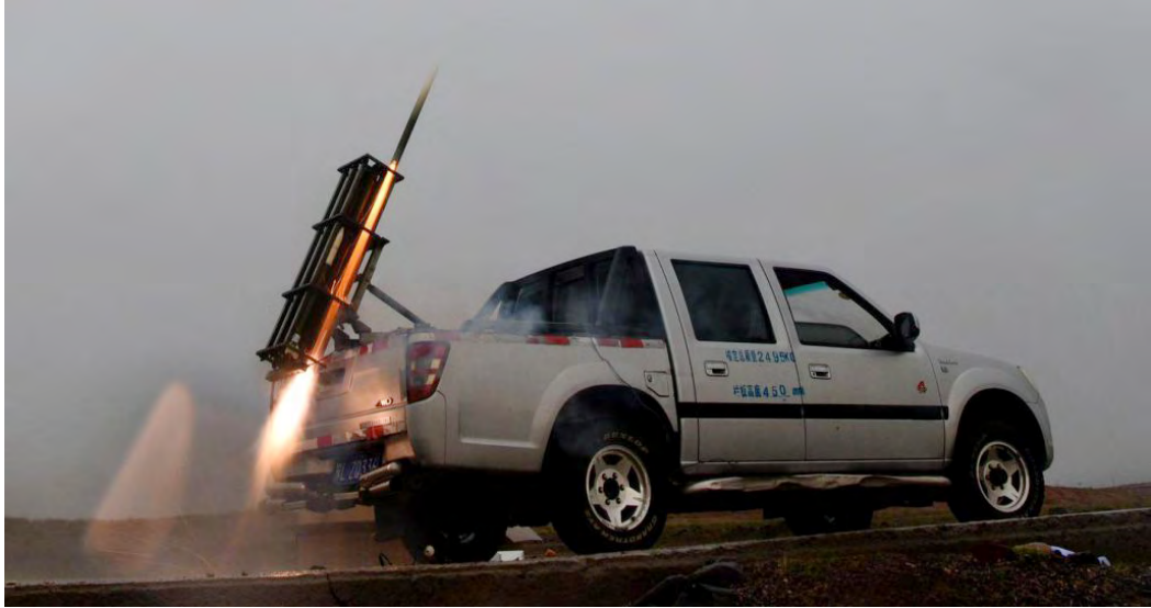
A cloud-seeding rocket launched to ease the drought in Bayannur, Inner Mongolia in July 2018. Scientists are testing such technologies to alter rainfall patterns. PC: China Dialogue .
