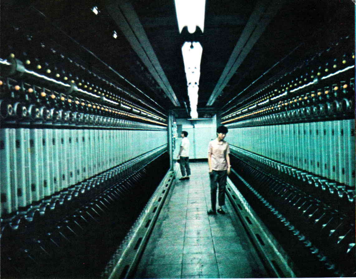
A forest of spindles in the terylene plant's long-fiber shop.
