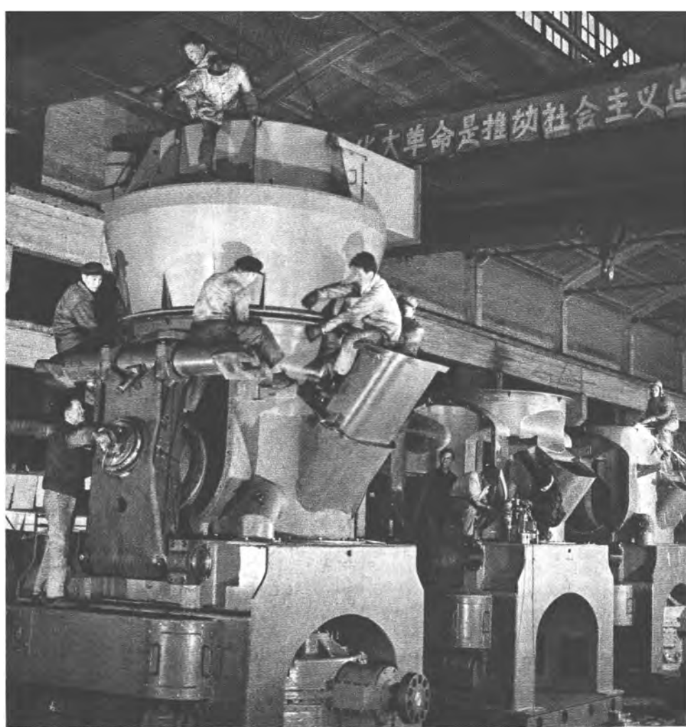
Workers of the Shanghai Metal Mining equipment Plant used indigenous methods to solve seven key problems in making this coal pulverizer with medium speed. The technology of processing the large helical bevel gear reaches advanced world level.
