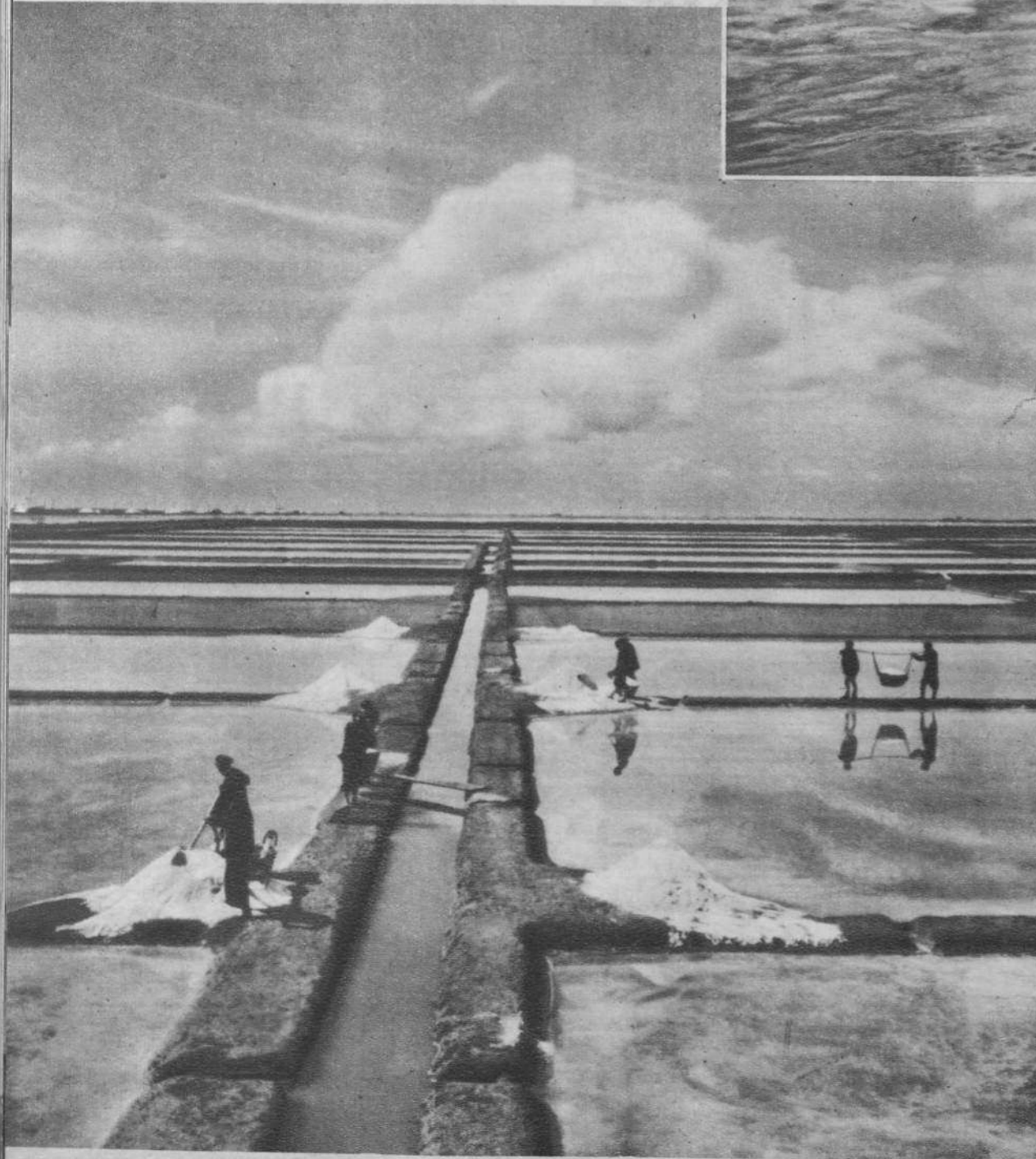
When the water in the reservoir has evaporated until its sodium chloride content has reached 5 per cent, more water is taken in and the process repeated
